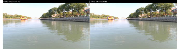
Fig. 3. Filter-free vs. Kalman tracking on the same detections. Without a motion model (left) a missed detection ends a track and it re-appears with a new identity, yielding 71 identities over the sequence; the Kalman tracker (right) coasts through brief dropouts and preserves identity, yielding 60.
